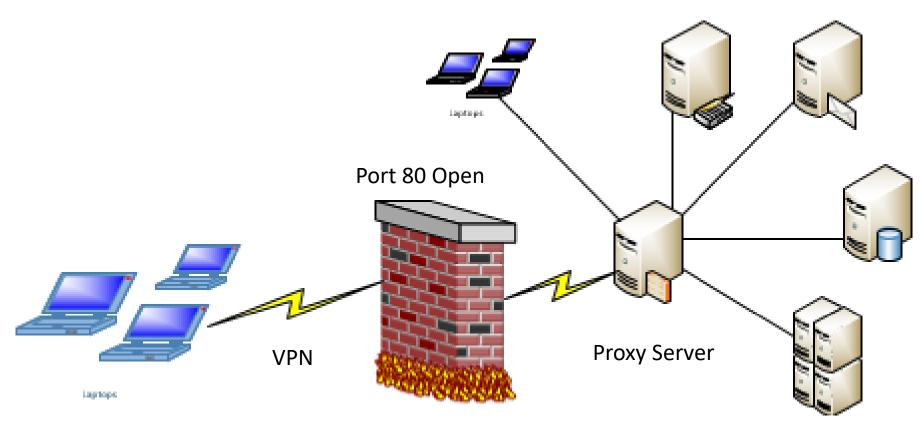
Prior to server hosting, PAAS, SAAS, etc., many datacenters were open networks internally. No segmentation or server connection restrictions and minimal ports open through the firewall. Any user connected must operate on a VPN or Citrix server.
